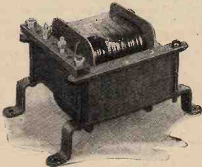
Heavy-duty choke for the "All D.C. Three," made by W. Bryan Savage.
