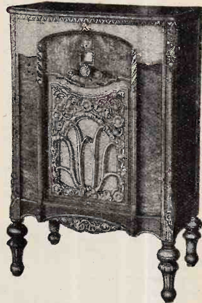
Amrad Rondeau receiver. There are four screen-grid valves, and a local-distance switch is included. Automatic volume control is used to prevent overloading.
