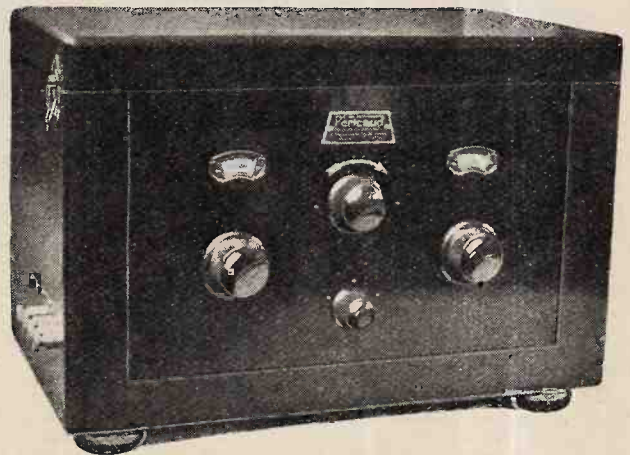
Péricaud E3 receiver with single screened H.F. stage and variometer plate coupling.
