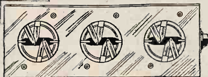
Ganged wave change switch action fitted in Colvern coils.
