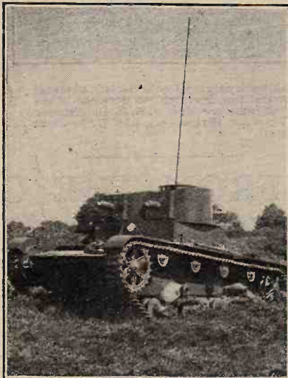
A TANK AERIAL. — This Vickers-Armstrong tank is equipped with a Marconi 8-metre transmitter, and the aerial consists of a flexible copper-plated steel rod, 12 feet high, which is almost invisible.
