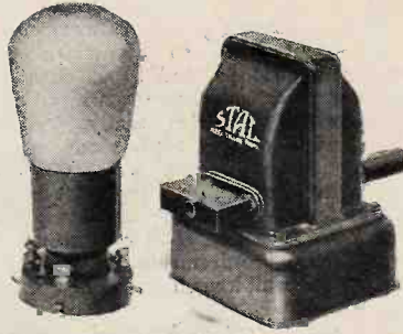
"Triotron" metal-coated detector valve and the "Stal" trickle charger.
