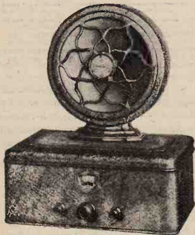
Crosley 26 H. receiver. A battery-operated set with three screen-grid H.F. valves and push-pull output.
