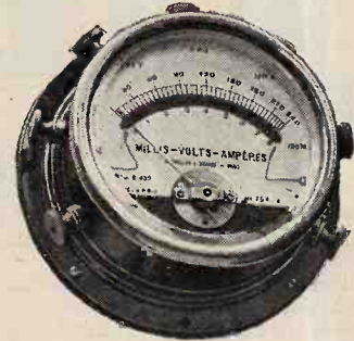
Cifel "Multi-meter," with moving coil movement and parallax mirror. (Fonteyn.)
